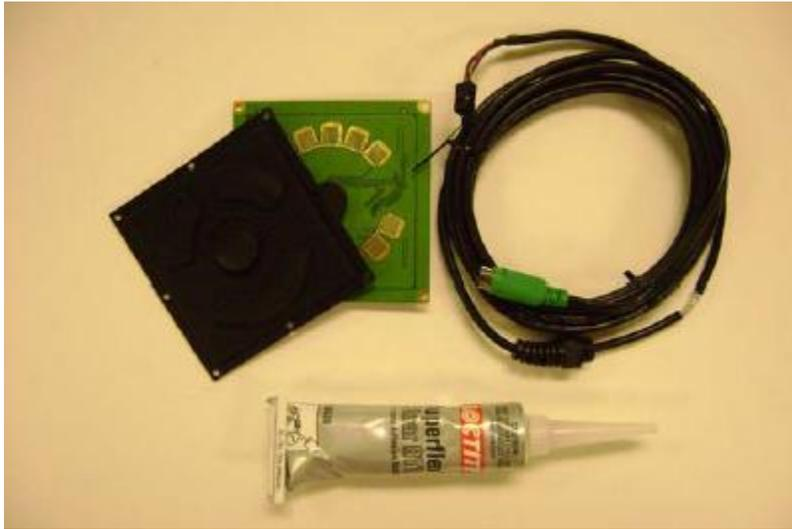
1. OEM Printed Circuit Board
