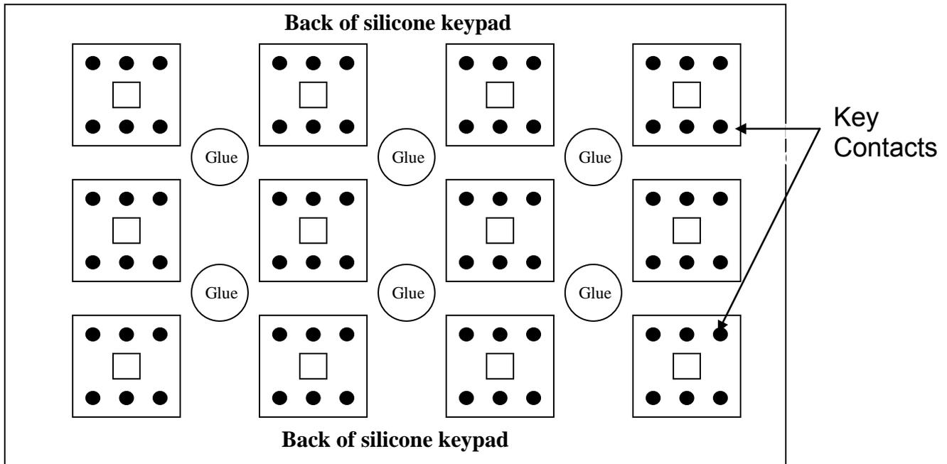
Apply silicone adhesive [Stealth recommends SuperFlex by Loctite] to back side of silicone overlay (keypad). Sparingly dab glue on the middle of each key intersection across the whole keyboard as seen in this picture. Also apply to inside of center portion of FingerTip Mouse pad (where the sensor/joystick lies) if OEM kit incorporates the FingerTip Mouse.
